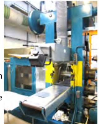
*The Fuel Fabrication Plant: Here, uranium powder was rolled out for fuel elements for the DR 3 reactor*
