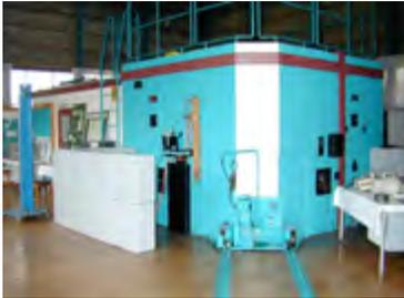
DR 1 – Danish reactor 1 was a so-called zero-power reactor (maximum 2 kW), thus the amount of radioactivity it contained was modest compared to reactors DR 2 and DR 3. The reactor was commissioned in 1957 and shut down in 2001.
