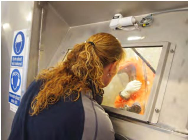
Waste which is only surface contaminated is cleaned in a decontamination cabin by sand- or glass-blasting. The cabin can be operated from the outside through a glove box or from the inside by an operator wearing a protective suit, if the item is too large and heavy to be handled through the glove box.
