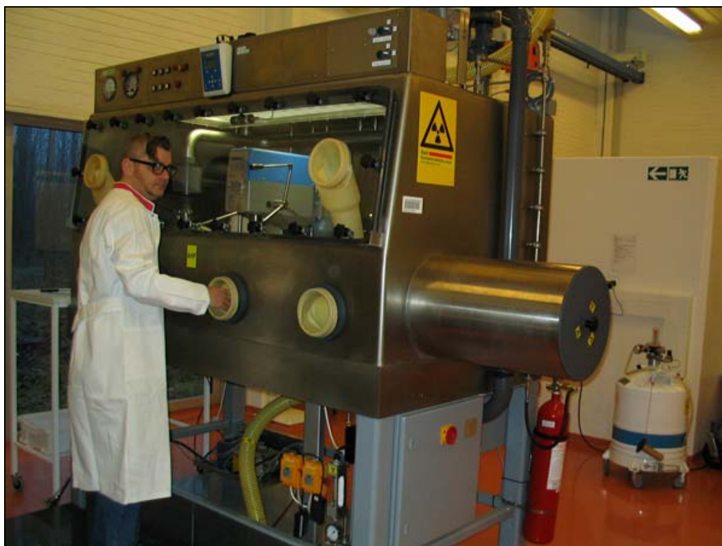
The glove box in the Radiation Laboratory is used for preparation of samples from the decommissioning.
