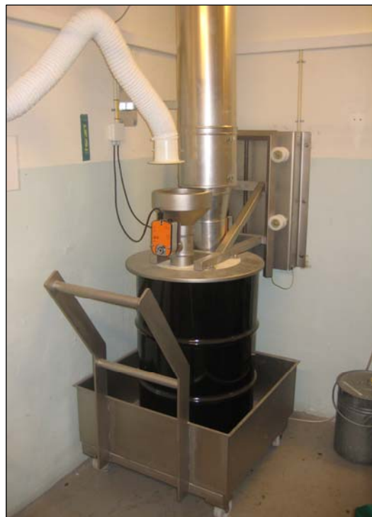
Organic liquids are dehydrated by use of a standard drum equipped with suction extraction.
