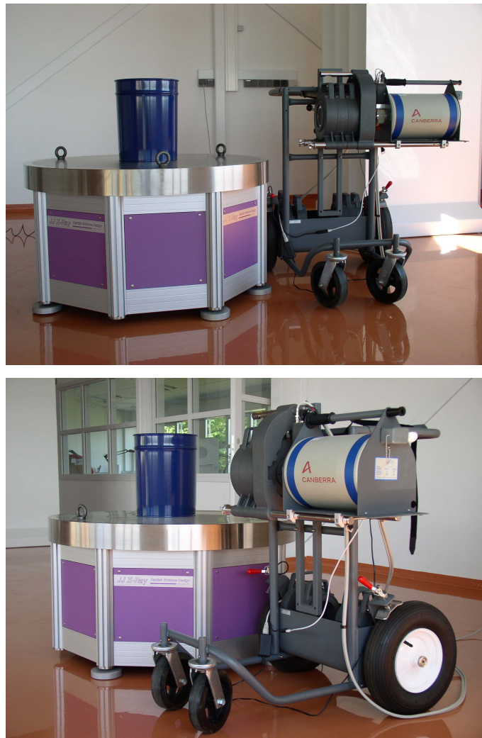
Figure 5. Germanium detector with a 100% efficiency relative to a 4×4 inch sodium iodide detector. The detector is surrounded by a circular lead shield of 50 mm thickness. The objects are placed on the rotation table in front of the detector.
