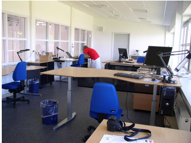
Figure 3. Control room at the Clearance Laboratory with computers connected to the germanium detectors in the measuring hall. Selection of measurement geometry, setting measuring time and all data processing of the measurements are carried out from the control room.
