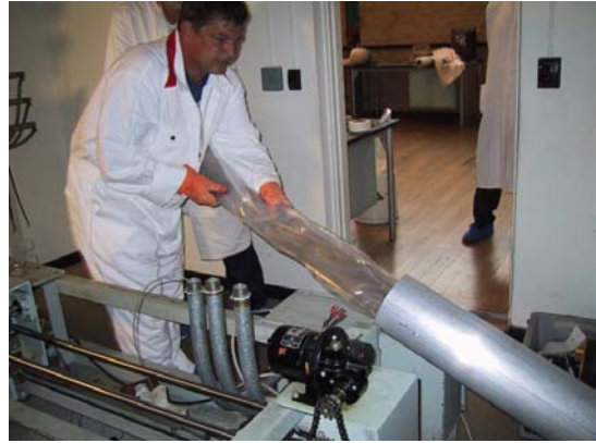
Figure 8 Transferring a control blade to the special container
