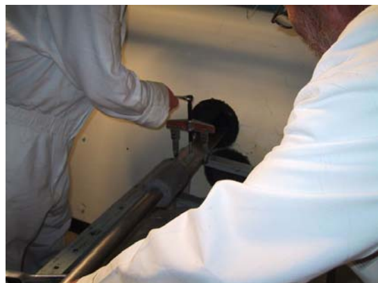
Figure 6 Removing the pin connecting the control blade to the guide rod
