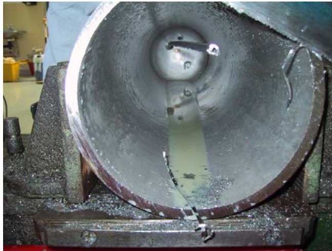
Figure 24 The Fuel Drain Tank cut apart
