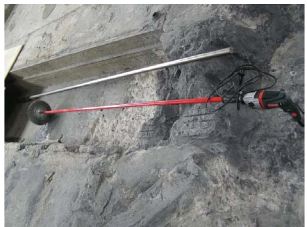
Figure 55 Tool for decontaminating the pipe
