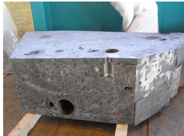
Figure 39 Free-releasable block after removal of the activated slab
