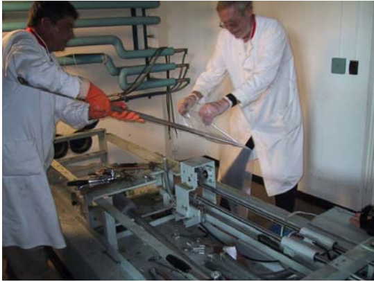
Figure 7 Transferring a control blade to a plastic bag
