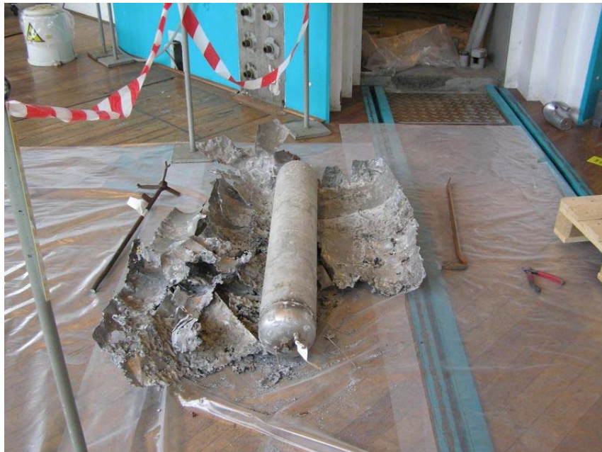
Figure 23 The Fuel Drain Tank
