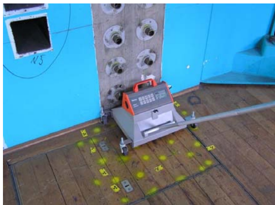
Figure 28 Contaminated area under the Fuel Mix Bowl
