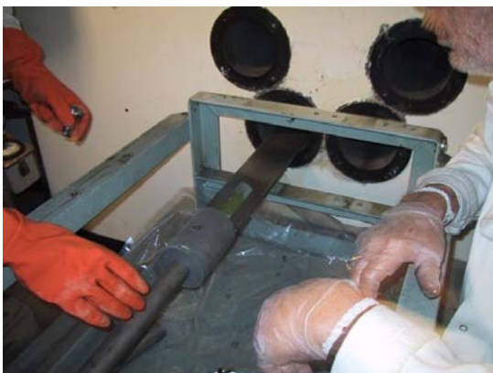
Figure 5 Control rod being pulled out
