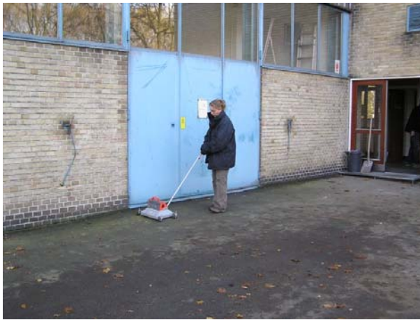
Figure 70 Measurement with contamination monitor north of the building
