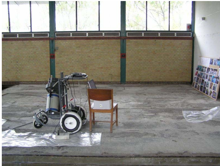
Figure 65 A Ge-detector set up for measurement on the upper part of the southern wall
