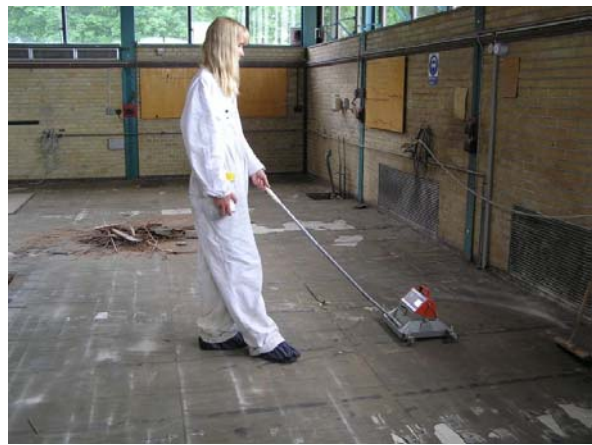
Figure 47 Control measurement of the layer below the wooden floor.
