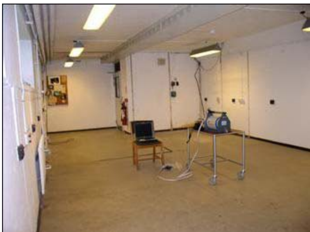
Figure 68 Ge-detector in the counting laboratory
