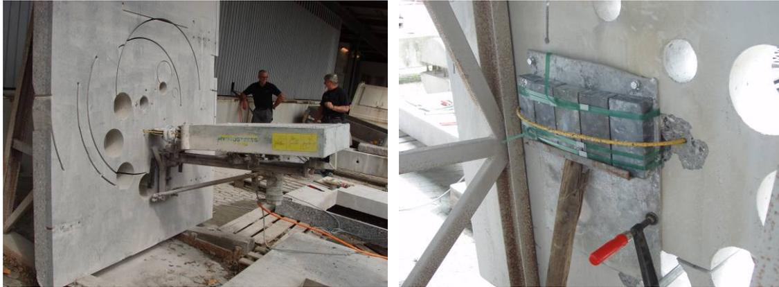
**Figure 57. Test structure set-up for a test cutting using wire.**
