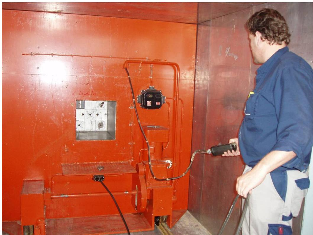
**Figure 13. The sliding door is run out. At the centre is the plug for removing graphite for the thermal column. The rail system can be glimpsed at the bottom.**
