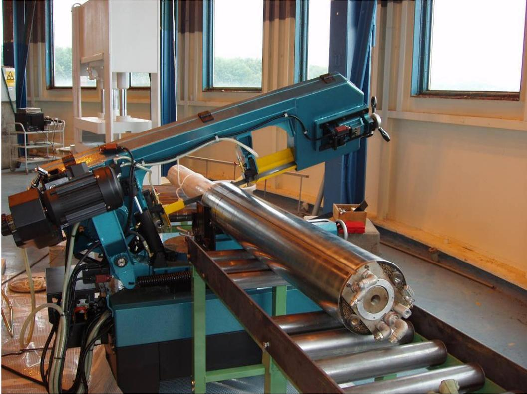
**Figure 23. Partitioning of a B-tube in an automated band saw.**
