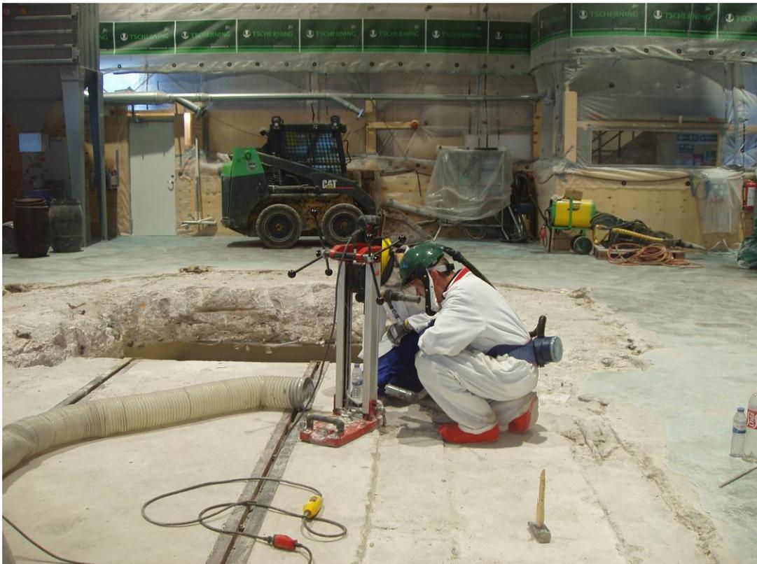
**Figure 68. Taking of drill samples from the concrete floor.**
