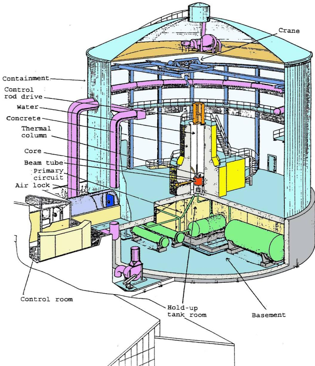
**Figure 2. Cross-section perspective of reactor DR 2 in the building.**
