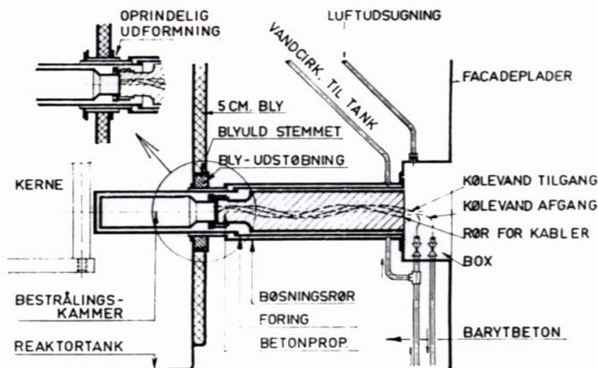
**Figure 18. Basic design of horizontal beam tubes.**
