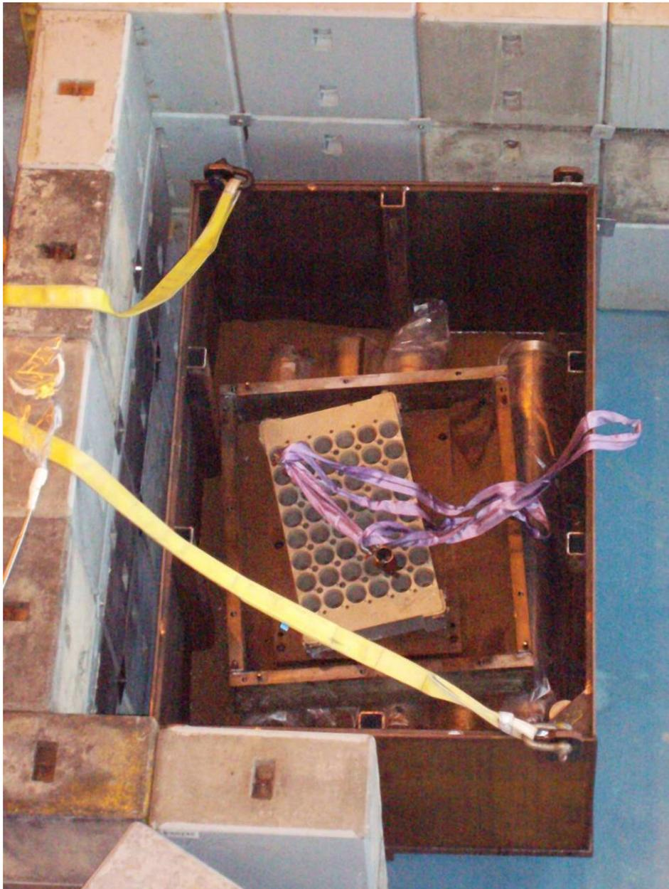
**Figure 34. The grid plate in the container before it was closed. The shielding box and plugs are barely visible at the bottom.**
