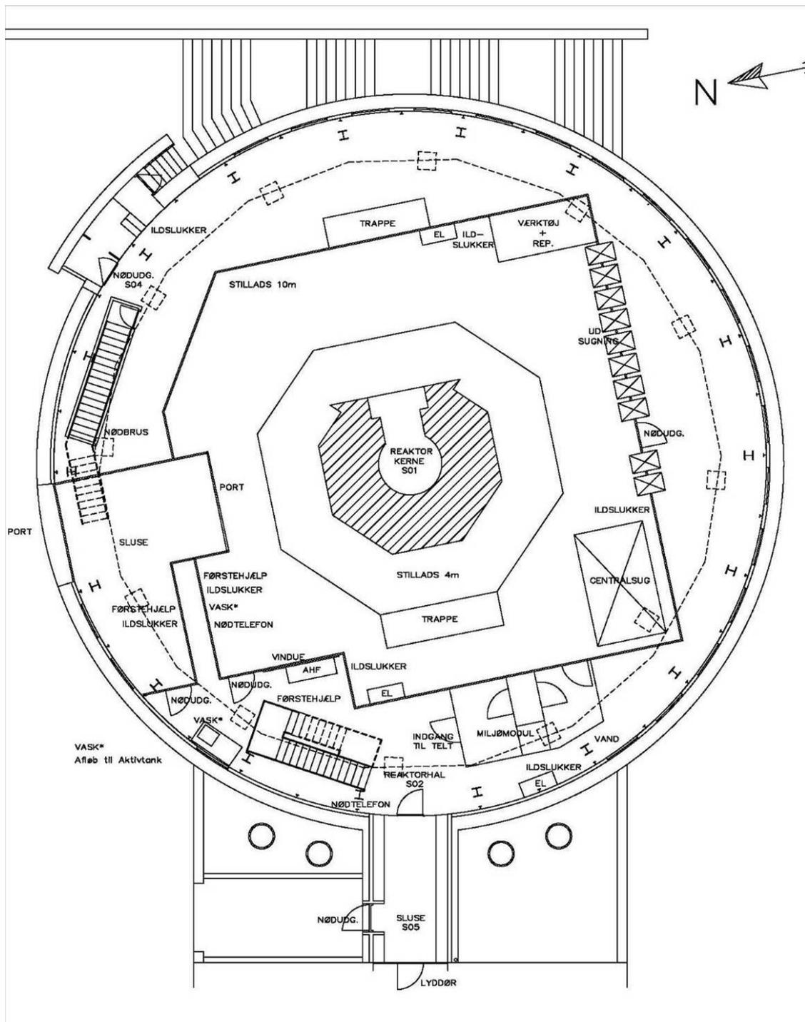
**Figure 44. Layout plan for tent in concrete demolition (process step 1).**
