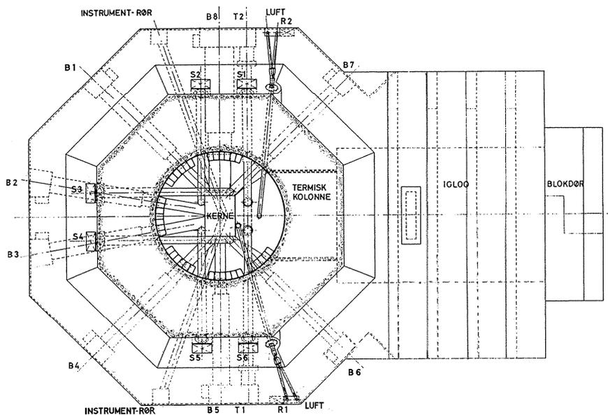
**Figure 15. Horizontal cross-section through reactor DR 2.**
