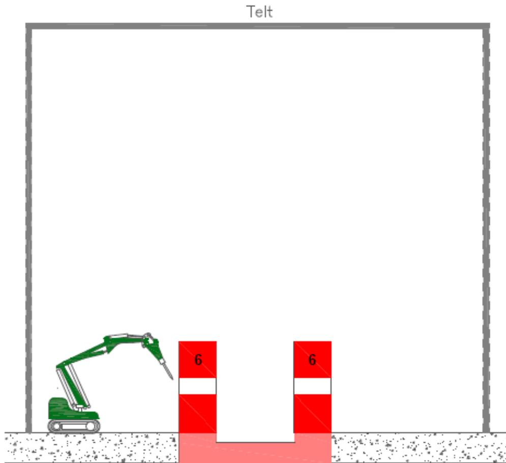
**Figure 64. Process step 6, Demolition of activated material from reactor block, lower part.**
