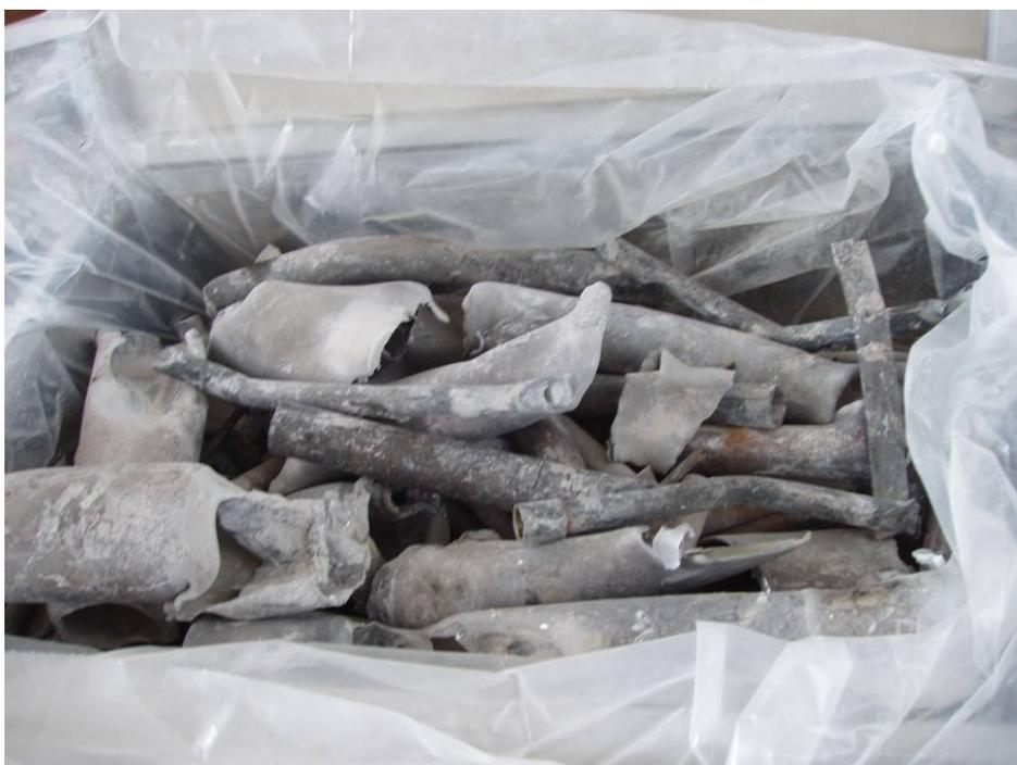
**Figure 70. Cast-in pipe sections from the concrete structure removed for further checks.**
