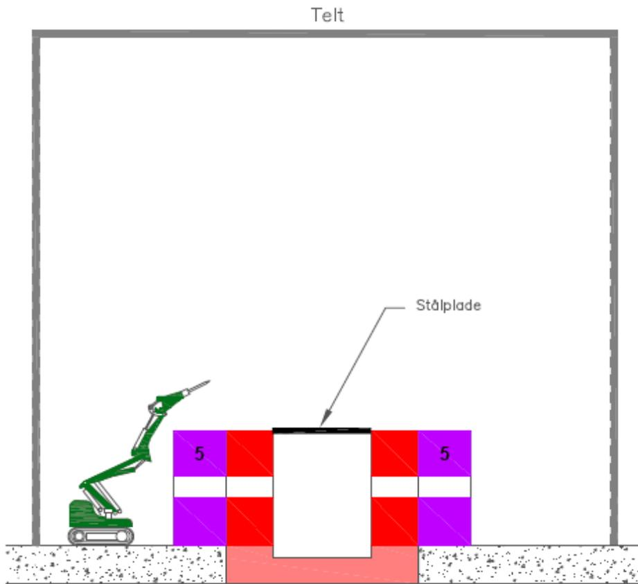
**Figure 62. Process step 5, Demolishing of non-activated material from the reactor block, lower part.**
