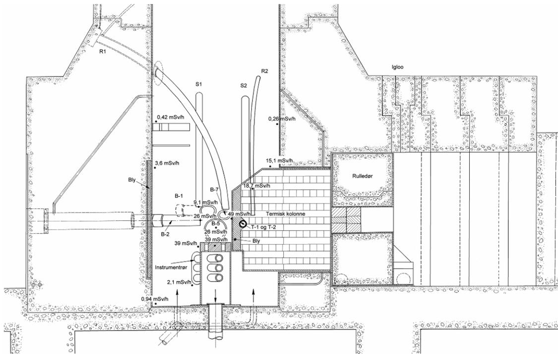
**Figure 5. Cross-section of reactor block and thermal column showing the radiation levels measured with TL-dosimeters in the spring of 2001.**
