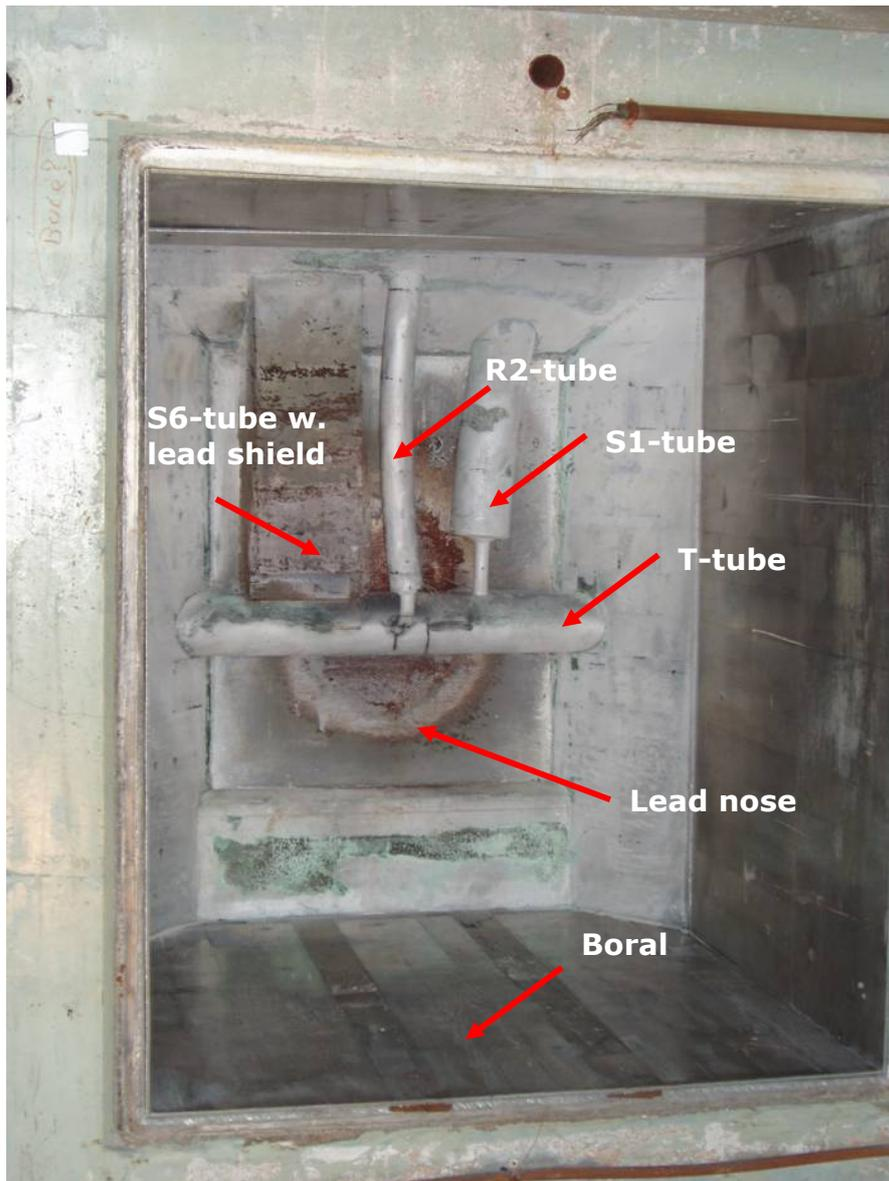
**Figure 28. Thermal column with the graphite removed and an uncovered lead nose (R1-tube covered by S6).**
