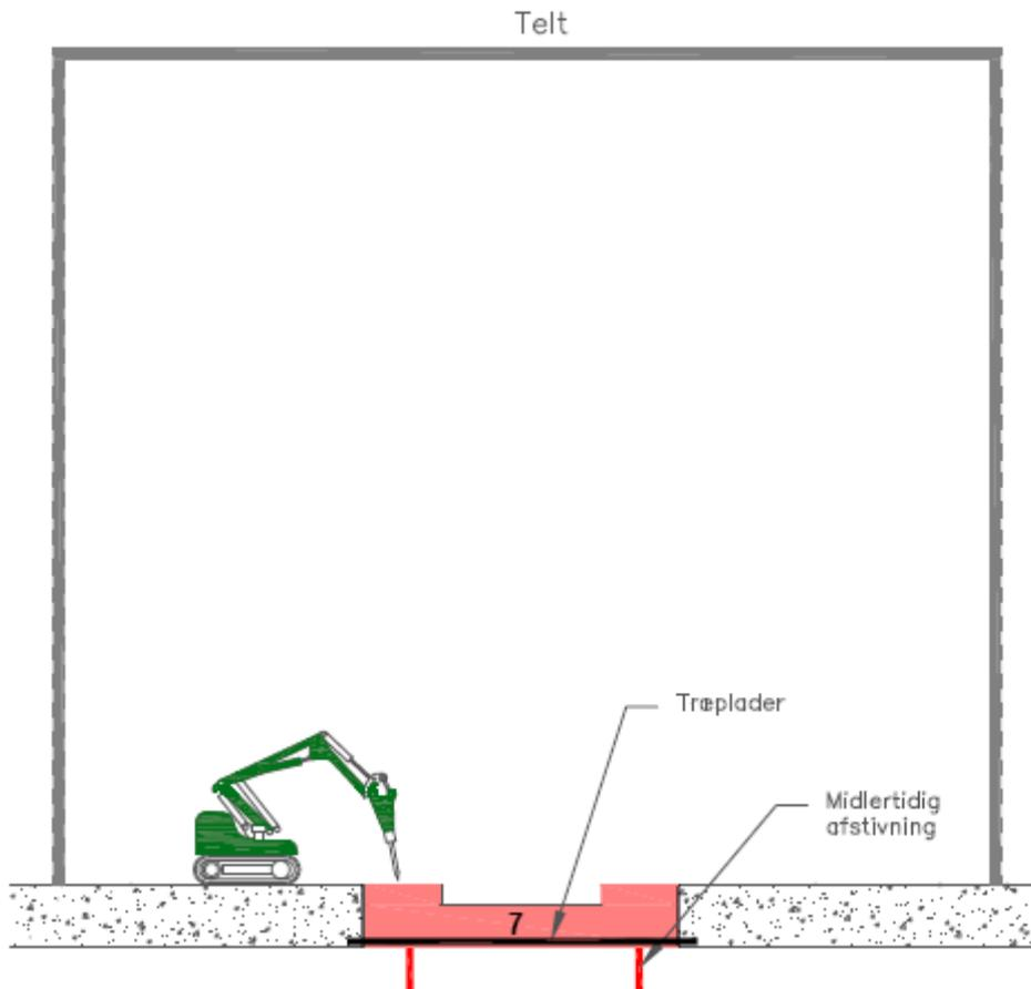
**Figure 66. Process step 7, Removal of activated concrete from floor.**
