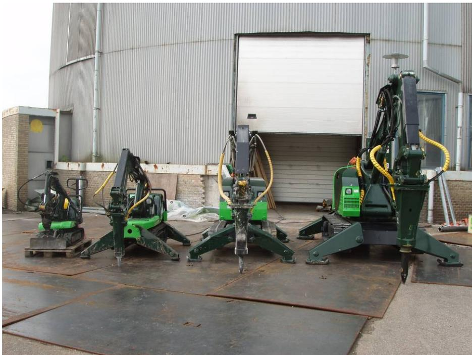
**Figure 50. Remote-controlled demolition robots of the 'Brokk' type; these were used for the assignment.**
