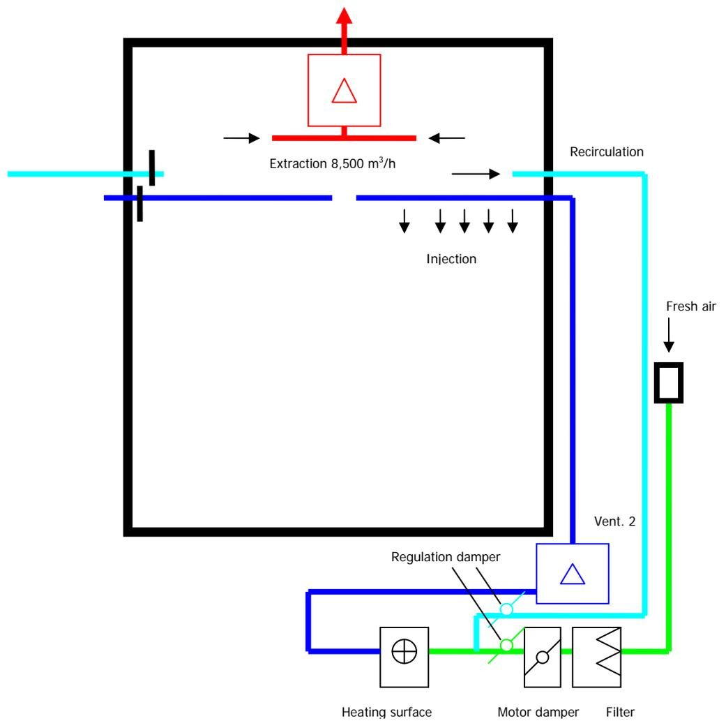
**Figure 10. Skeleton diagram of new ventilation system**
