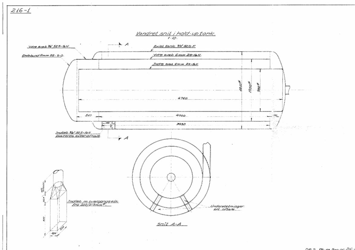
**Figure 37. Decay tank, cross-section.**
