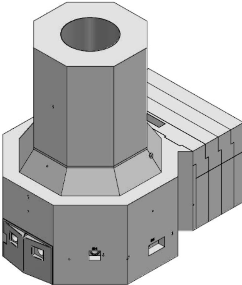
**Figure 3. Elevated view of the DR 2 reactor's biological shield.**
