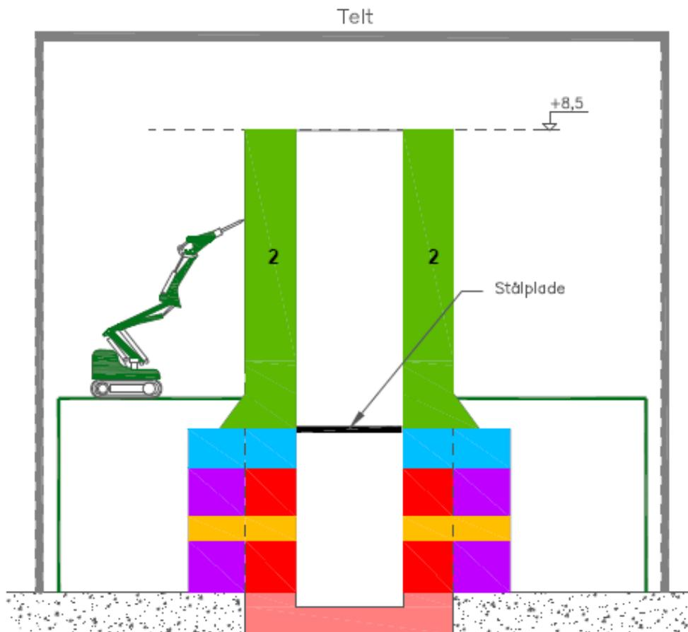
**Figure 51. Process step 2, demolition of non-activated superstructure (chimney).**
