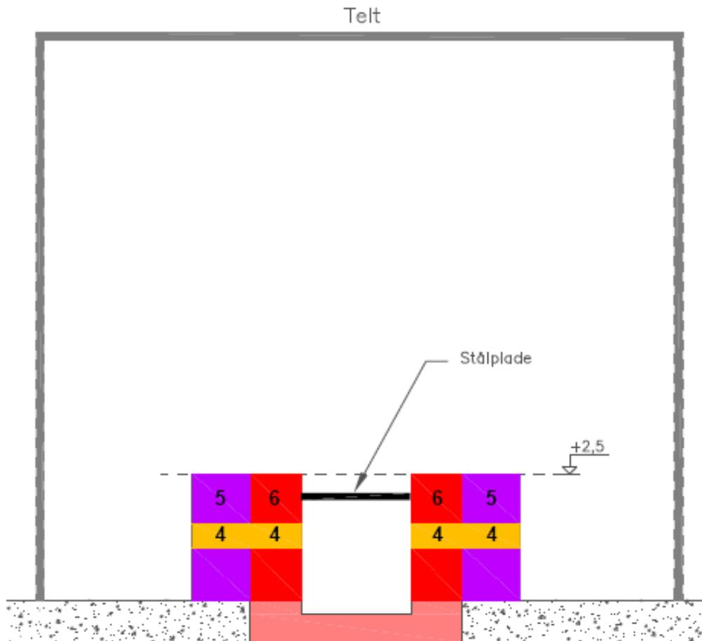
**Figure 60. Process step 4, Removal of activated lead-ins in the concrete.**
