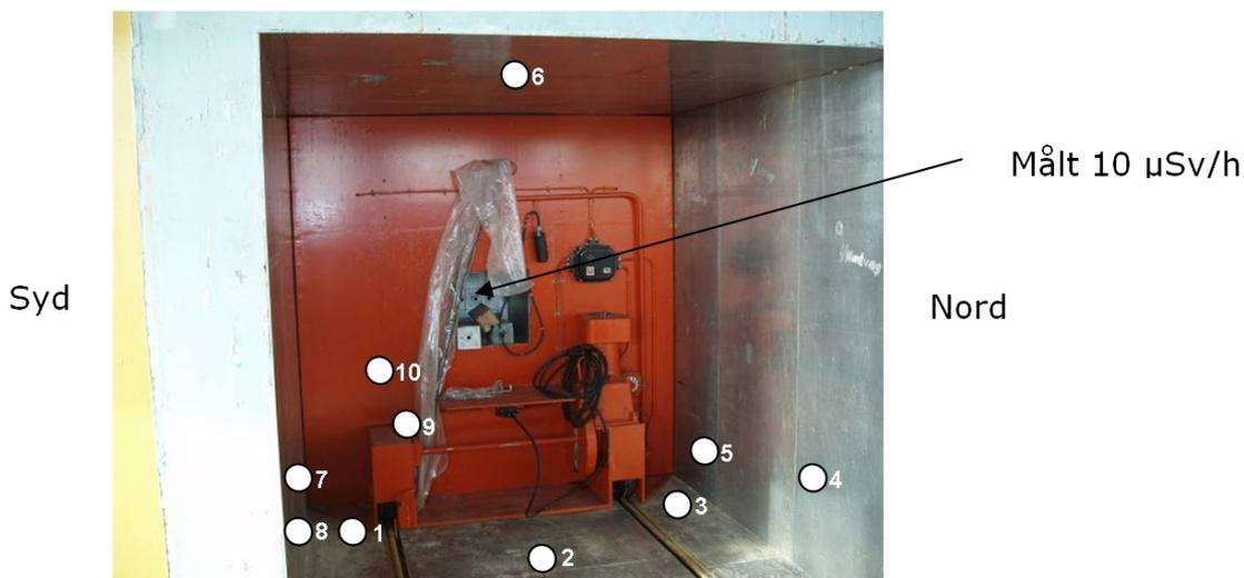
**Figure 14. Measurements in the igloo before the sliding door was removed**
