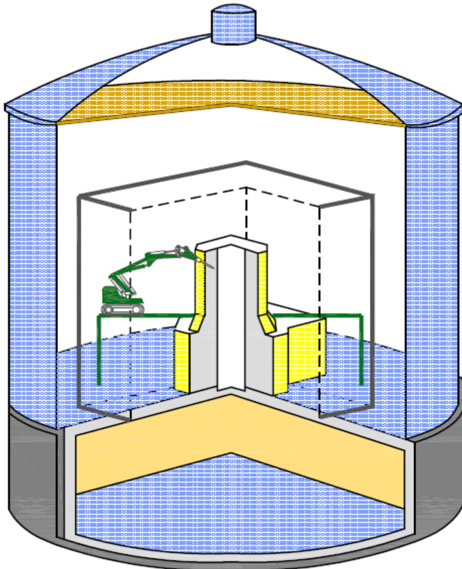
**Figure 48. Basic work site layout for concrete demolition.**
