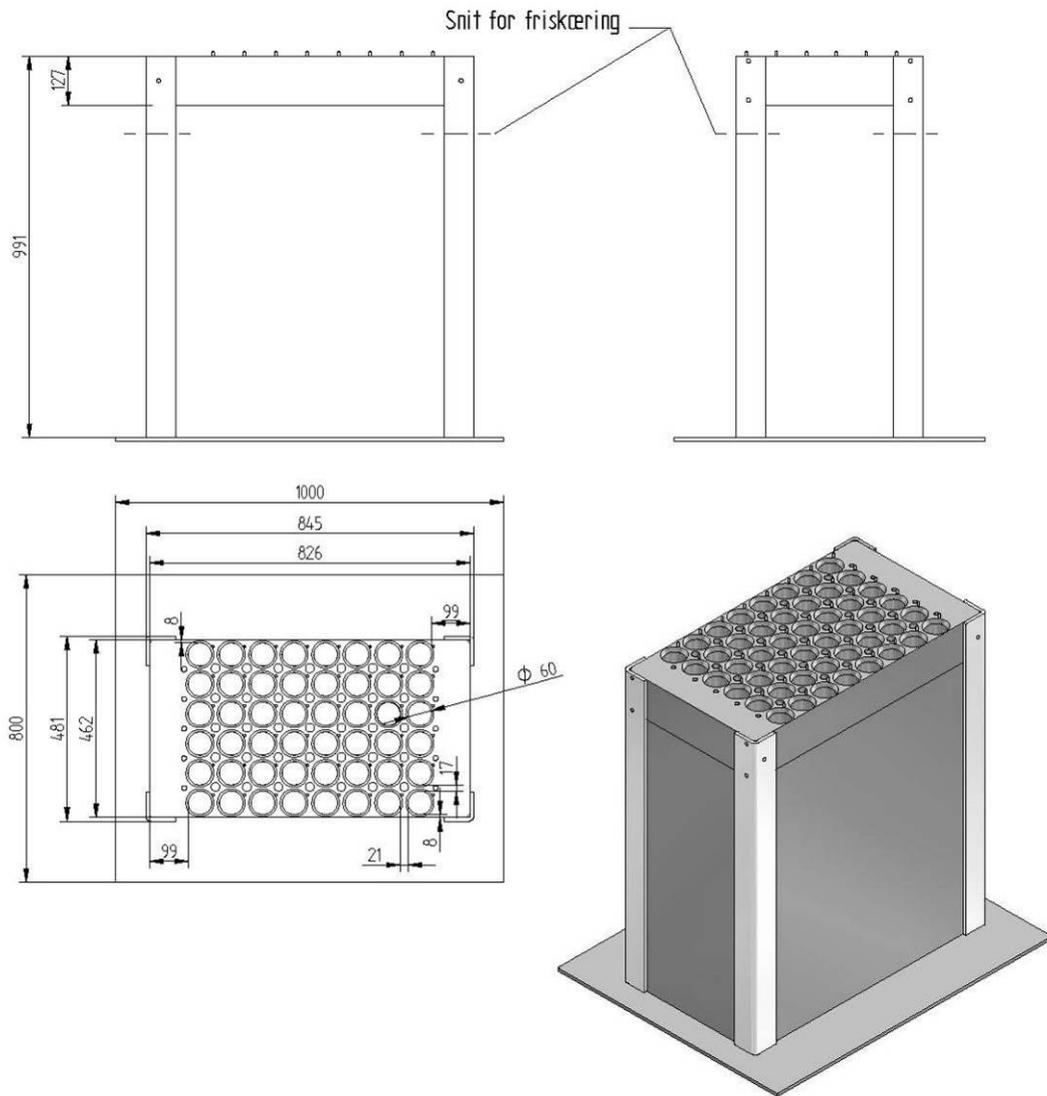
**Figure 32. Grid plate with rack and cutting points indicated.**
