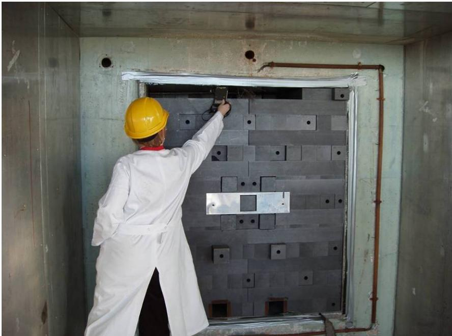
**Figure 24. Thermal column with graphite; radiation level is measured.**
