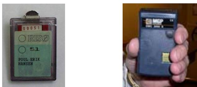
**Figure 73. TL dosimeter and electronic dosimeter**
