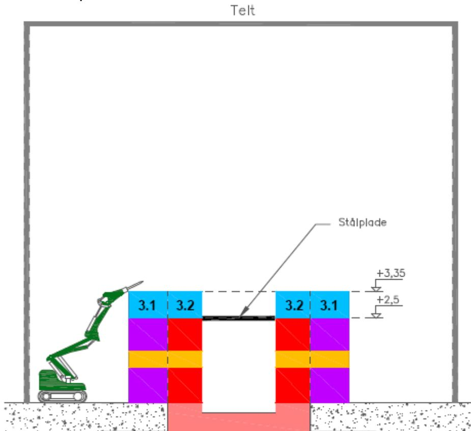
**Figure 54. Process step 3, Demolition of non-activated material from the reactor block, upper part (down to elevation level +2.5).**
