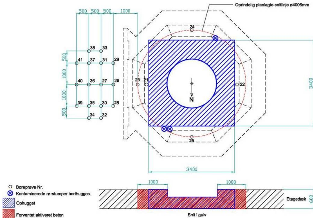
**Figure 69. Plan for drill core samples for checking the concrete break-down.**
