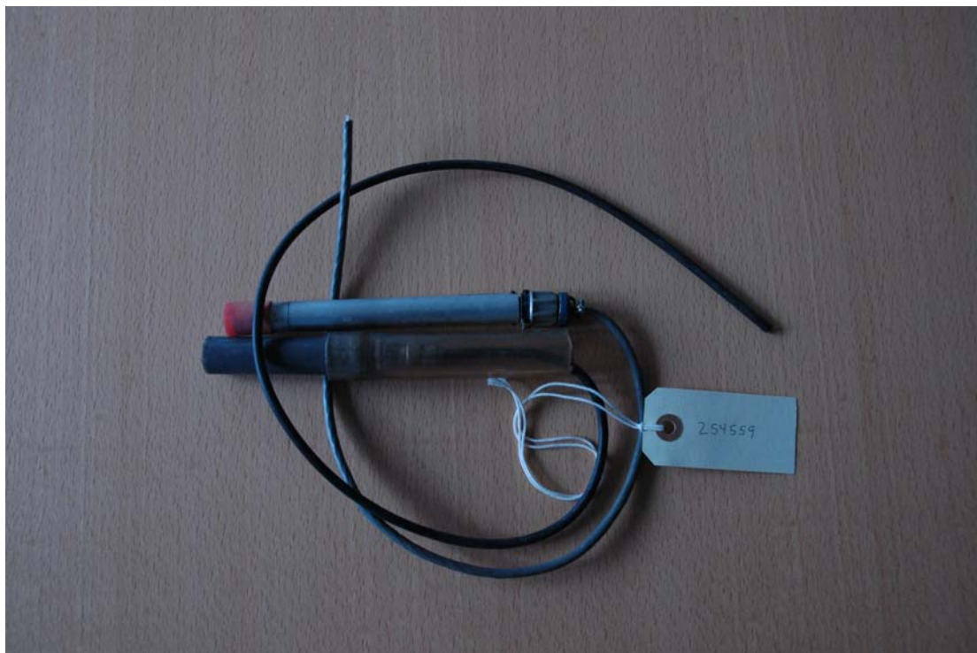
Figur 60. Prober for \gamma -detektorer.
